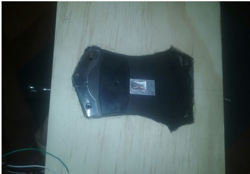
Figure 26: Optical PS2 mouse
